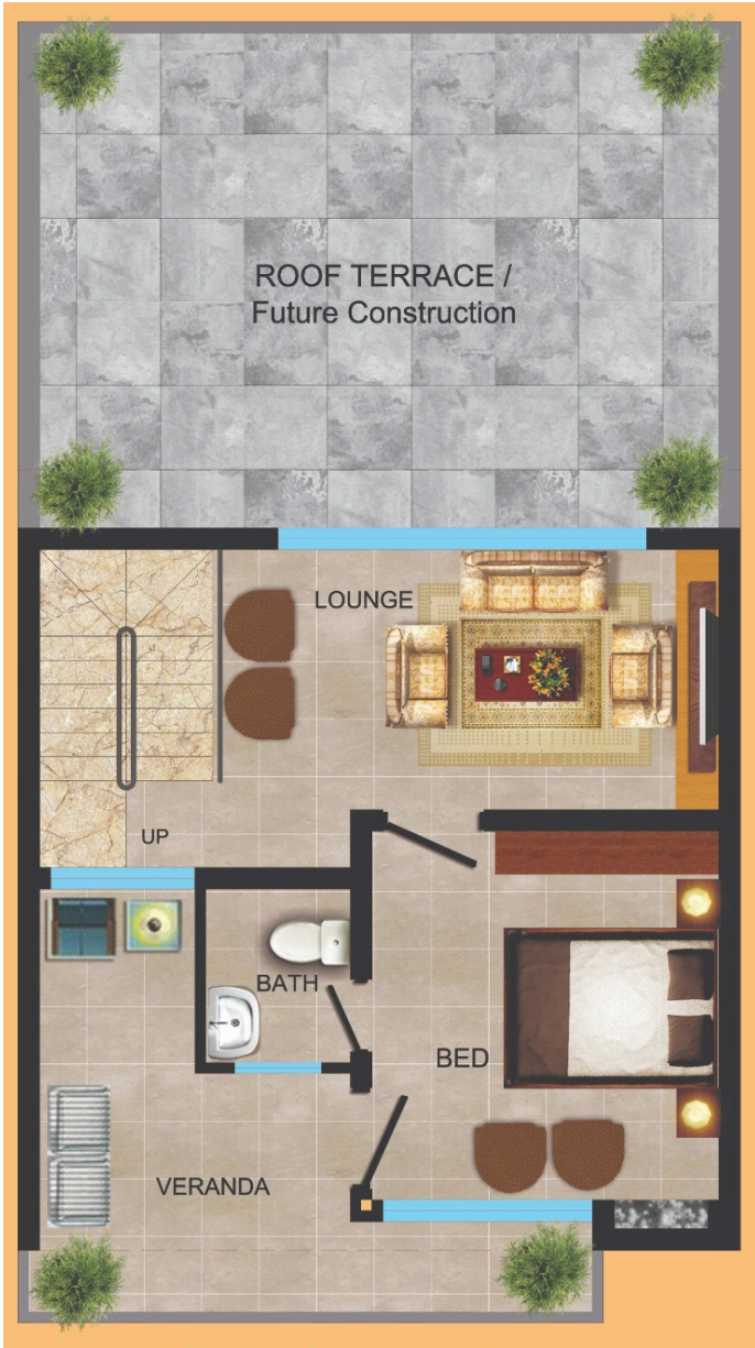
Proposed Design of a House..(25x50) Type-1 First Floor Plan Covered Area..625 sqft
