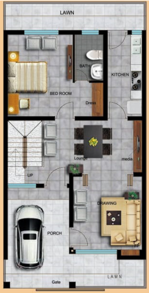
Proposed Design of a House..(25x50) Type-1 Ground Floor Plan Covered Area..1000 sqft
