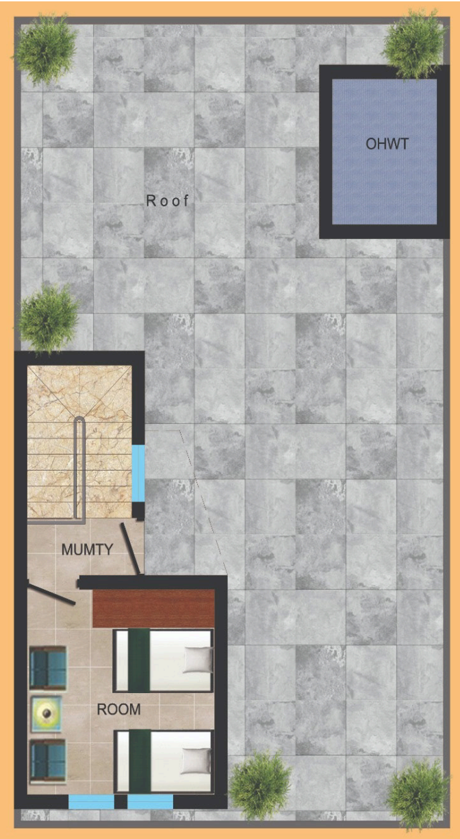
Proposed Design of a House..(25x50) Type-1 Mumty Floor Plan....250 sqft
